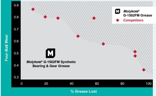
Figure 1: Molykote® G-1502FM Grease minimizes wear scar and grease loss
